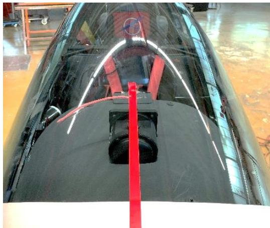
To do this, determine the center of the canopy with the help of adhesive tape or a thin thread.
