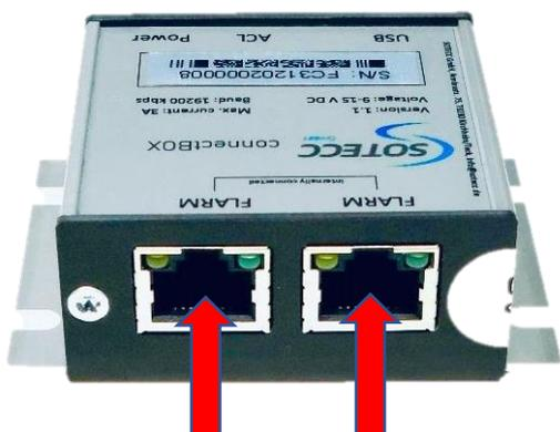
Finally, connect the FLARM® to the connectBOX with RJ45 or RJ12 cable. Both connections can be used. If no other device is connected which requires FLARM data, one port remains free. The two RJ ports of the connectBOX are connected internally, so it can also be used as a splitter (for looping through). The pin assignment corresponds to the "IGC GNSS FR Specifications". 8-pin (RJ45) or 6-pin (RJ12) connectors can be used without restriction.
