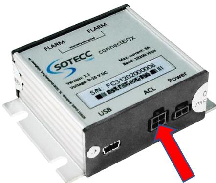
Plug the 4-pin Molex connector into the ACL slot of the connectBOX. Attach the ferrite core to the cable approx. 10cm in front of the connectBOX.
