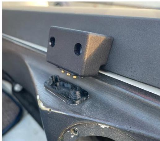
Drill through the template into the ventilation with a 2.5mm drill bit, then fix it temporarily with the screws supplied. Mill out the oblong hole of the template. If no cutter is available: drill out the outside with 7mm and the inner larger hole with 10mm, if necessary grind with a round file to fit. Then unscrew the template and dispose of it.
