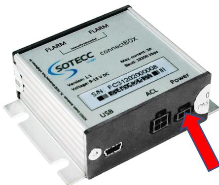
Connect the ConnectBOX via the supplied fuse/switch combination with the red/blue twisted 2-pin cable (power slot), adjust cable length if necessary. Then connect the switch to a free **and suitable** slot of the aircraft electrical system. Detailed overview: [see Appendix 1 \(Wiring\)](#).
