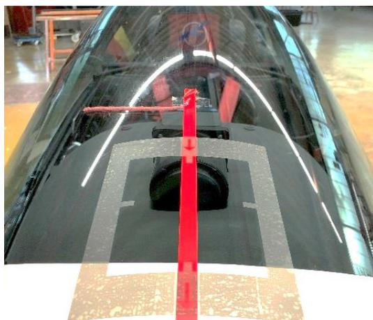
Before attaching the canopy flash, clean the canopy thoroughly with a suitable cleaning agent.
