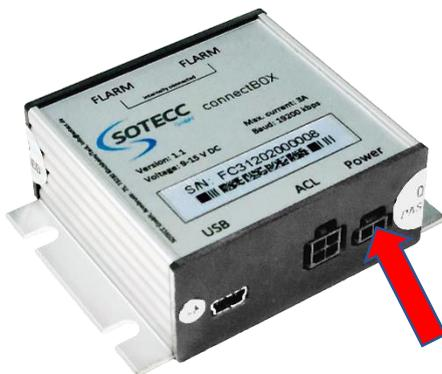
Connect the ConnectBOX via the supplied fuse/switch combination with the red/blue twisted 2-pin cable (power slot), adjust the cable length if necessary. Then connect the switch to a free and suitable slot of the glider onboard electrical system. Detailed overview: [see attachment \(wiring\)](#).
