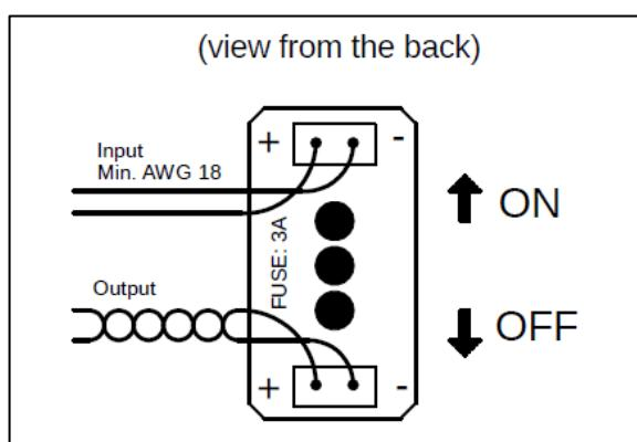
Drill a 6mm hole at a suitable location in the I-board. Cut the cable to length and connect it to the switch. Observe polarity at the switch. Connect plus+ (red cable) on the left side. We recommend the use of wire end ferrules.
