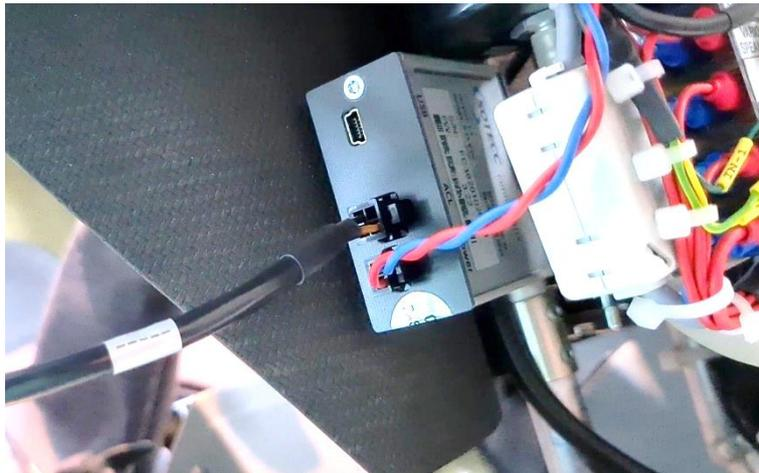
Finally, connect the FLARM® to the connectBOX with RJ45 or RJ12 cable.
