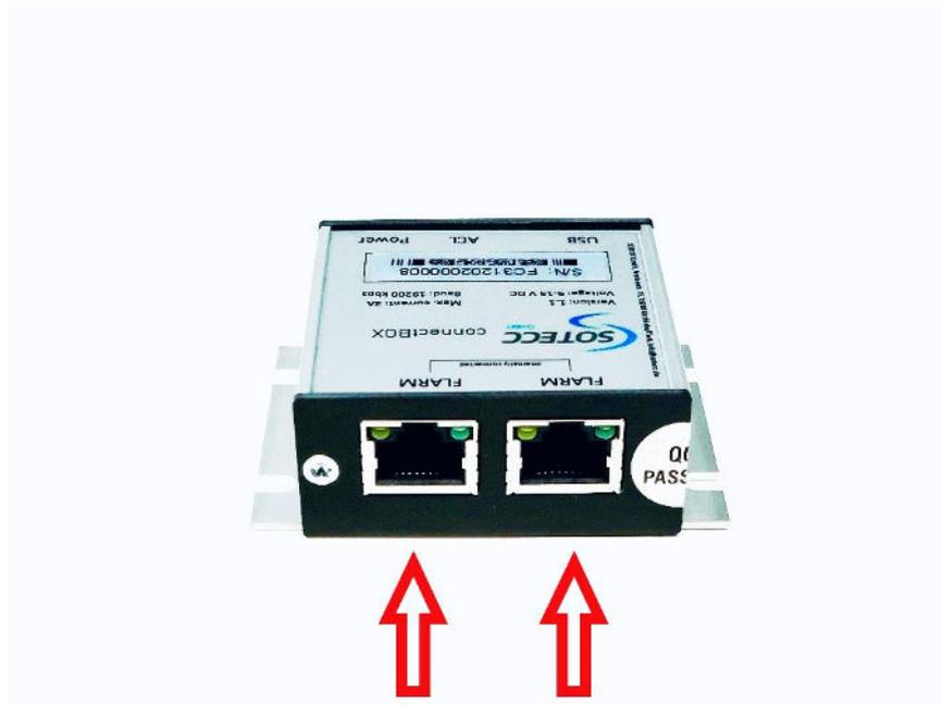
The ADS-B receiver TRX-1090 "Bluebox" cannot be connected between FLARM and the connectBOX. If necessary, connect the FLARM directly to the connectBOX.
