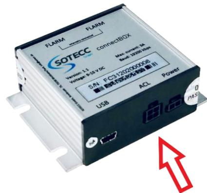
Connect ConnectBOX to a free fuse (3-5 A) of the glider's electrical system with the red/blue twisted 2-pole cable (power slot), adjust cable length if necessary. The switch for manually switching off the stub can be placed between the power cable.
