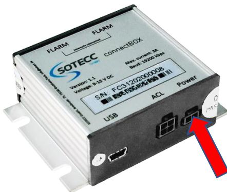
Connect the ConnectBOX via the supplied fuse/switch combination with the red/blue or black twisted 2-pin cable (power slot), adjust the cable length if necessary. Then connect the switch to a free and suitable slot of the glider onboard electrical system. Detailed overview: [see attachment \(wiring\)](#).
