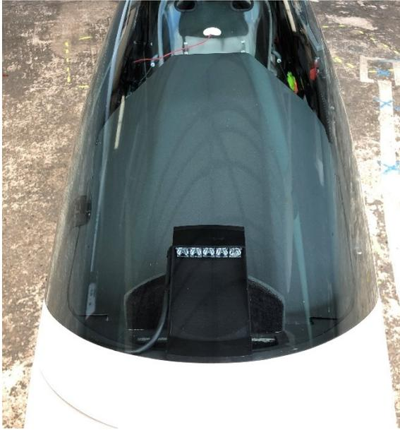
Tilt the canopy flash slightly downwards at the back so that only the outer adhesive strip touches the canopy. Then, starting from the front, carefully press down the adhesive surface that way that no air bubbles appear. Finally, press everything down firmly.
