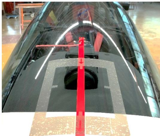
Before attaching the canopy flasher, clean the canopy thoroughly with a suitable cleaning agent.
