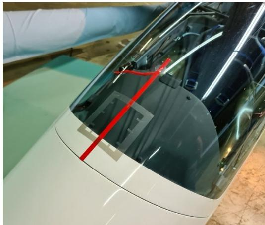
The front spacers of the template must be placed approx. 1mm behind the paint edge (towards the tail unit).
