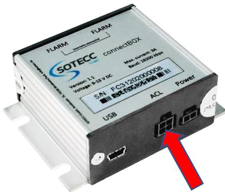
Connect the 4-pole cable of the counterpart (in the I-board cover, see work step 4, last picture) to the ACL slot of the connectBOX.
