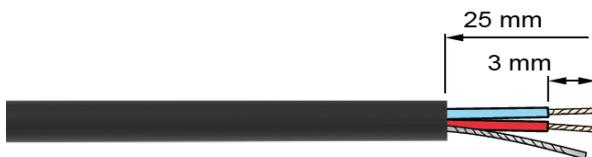
Unscrew the two TX8 screws from the canopy contact. Take out the spring contacts with holder. Push the cable through the hole in the side of the canopy contact. Then solder as shown, insulate with heat-shrink tubing and screw back to the canopy contact.
